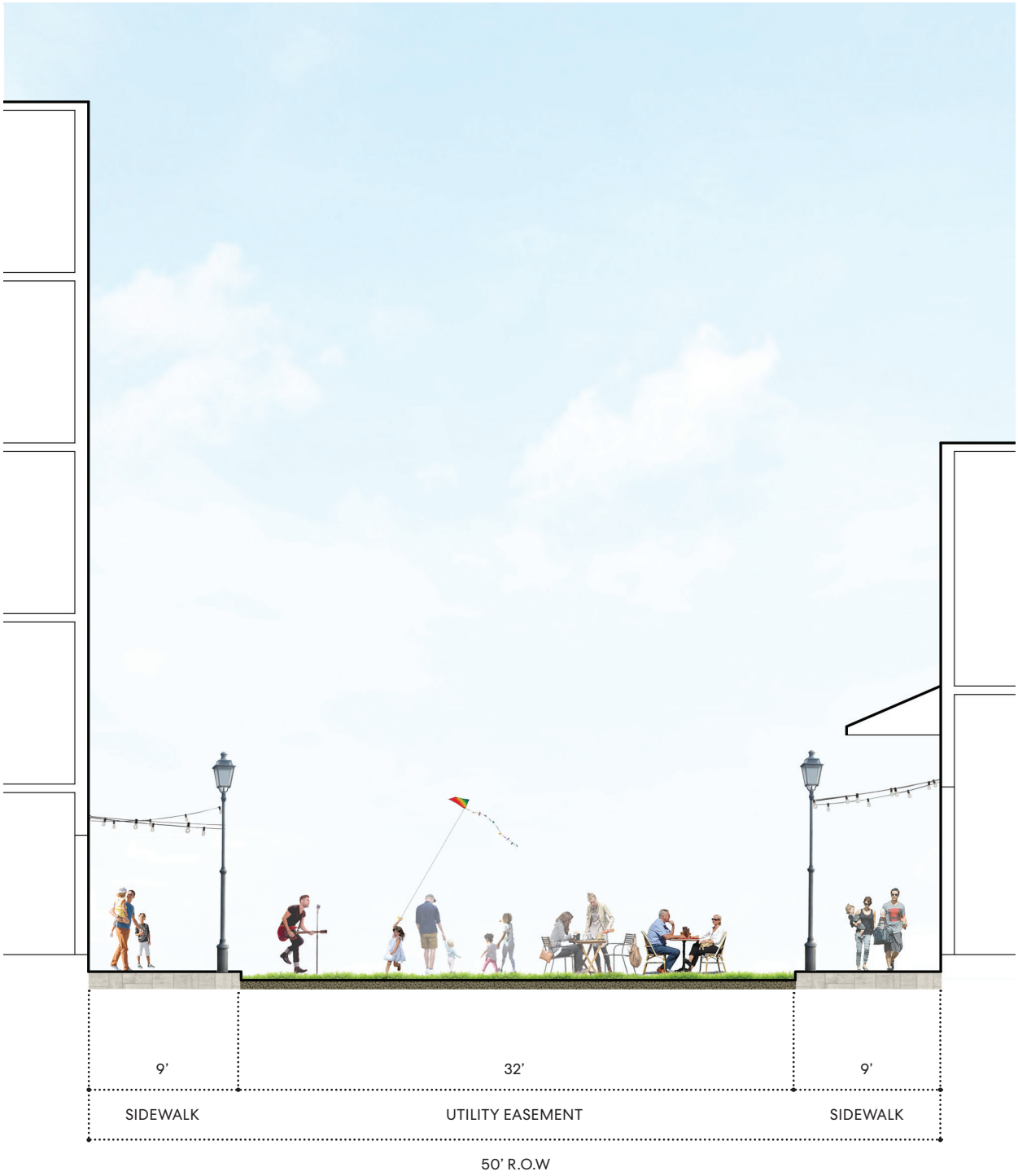
Section 10: North Area Utility Easement - Paseo Condition
